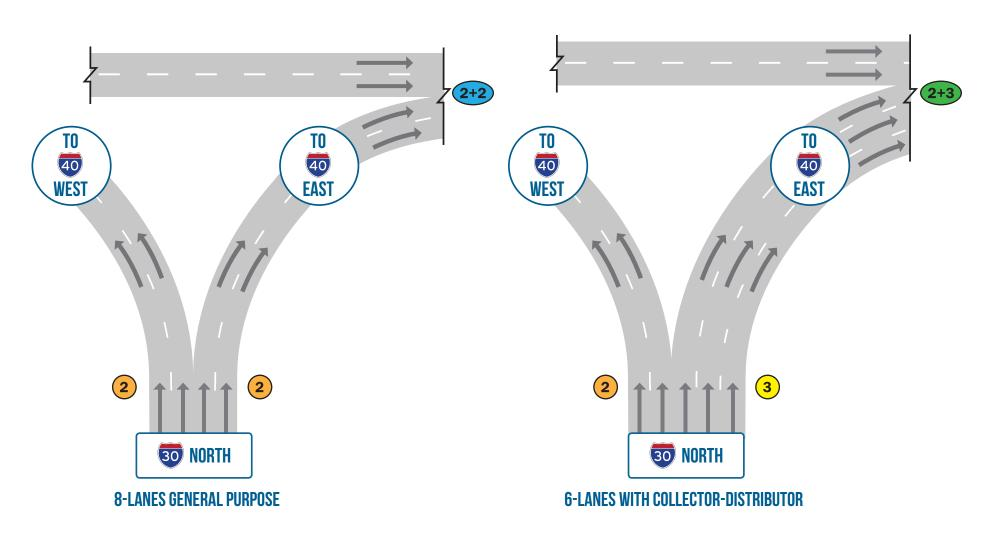
The issue is also compounded by the direct merges at the Cantrell interchange and Broadway on-ramps in the 8-Lane General Purpose Alternative.
